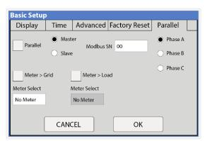
Figure 35: Parallel setup tab
