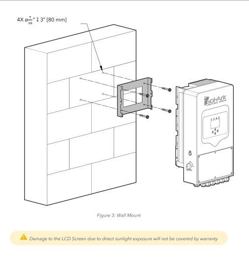
H. Mount the inverter in the optimal orientation as shown below.
