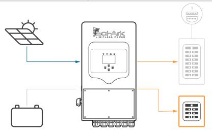
Figure 29: Limited Power to Load + Grid Sell
