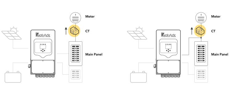
Figure 15: Installation of CTs for a) back-feed breaker and b) line side tap
