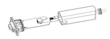
Figure 36: Connecting Wi-Fi dongle to ethernet
