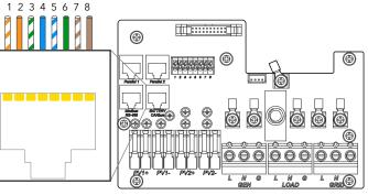
Figure 32: RJ-45 port configuration
