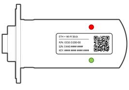
Figure 40: Wi-Fi dongle LED indicators
