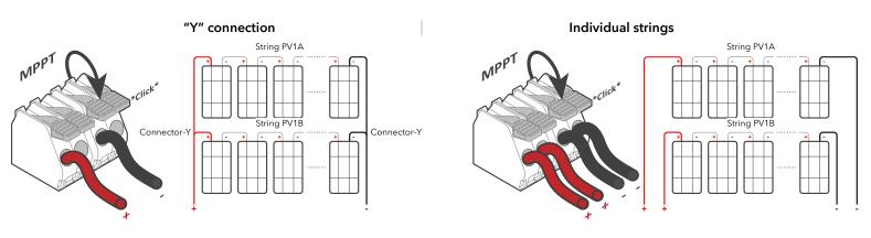
Figure 8: MPPT wiring and PV connections
