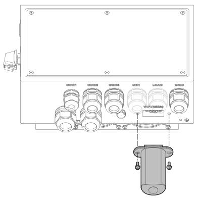
Figure 37: Connecting Wi-Fi dongle to Sol-Ark 5K-1P-N
