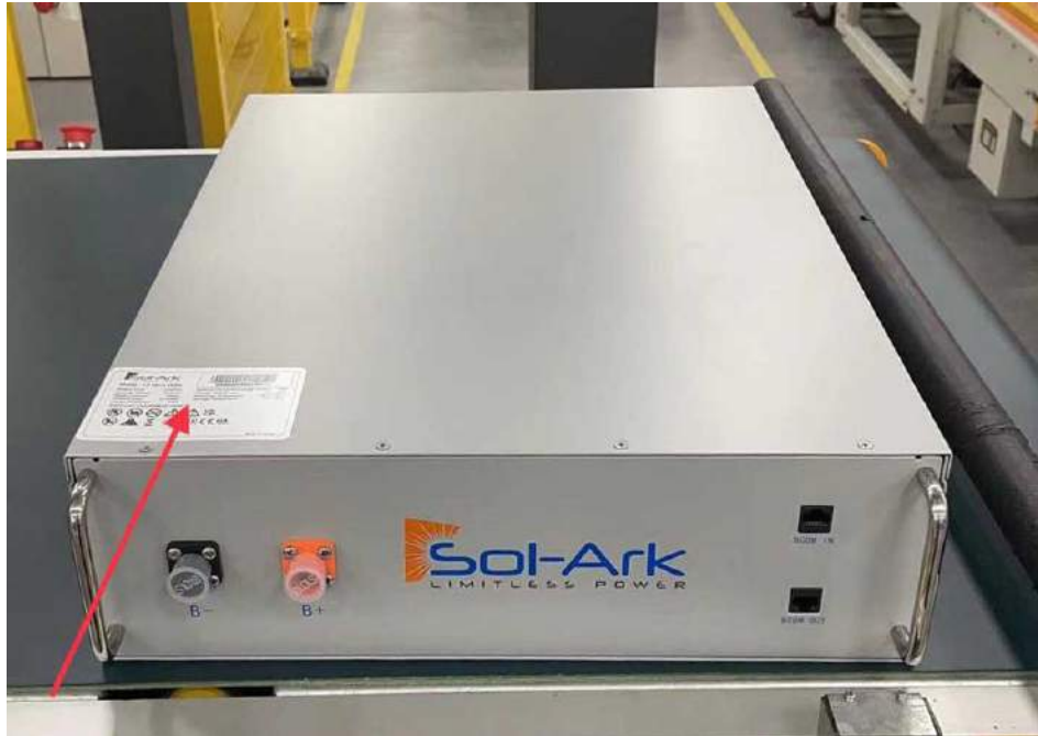
Figure 3: External View the L3 HV Battery Module
